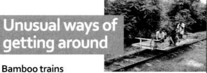
This is the best way to see rural Cambodia. A bamboo train, or nori as the locals call it, is a bamboo platform on wheels which travels along tracks. It's powered by an engine, and it can reach a speed of 40 kilometres per hour. Passengers sit on a grass mat on the nori. Noris may not be as comfortable as conventional trains, but they're certainly a lot cheaper. Pick up a nori from Battambang Station, but remember to agree on a price before you get on.
