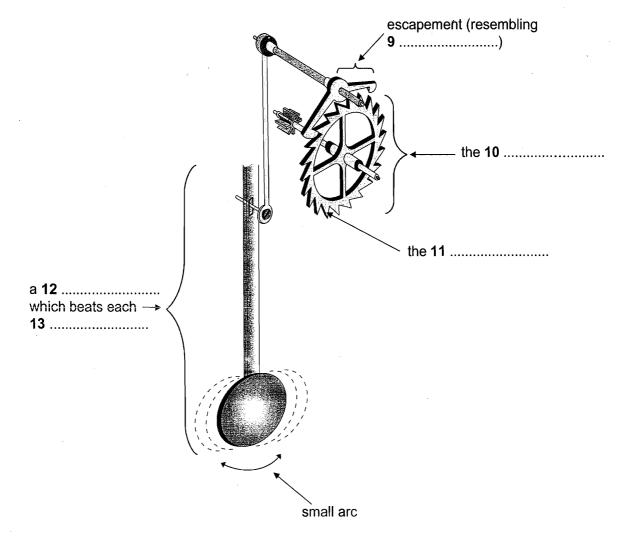
How the 1670 lever-based device worked
